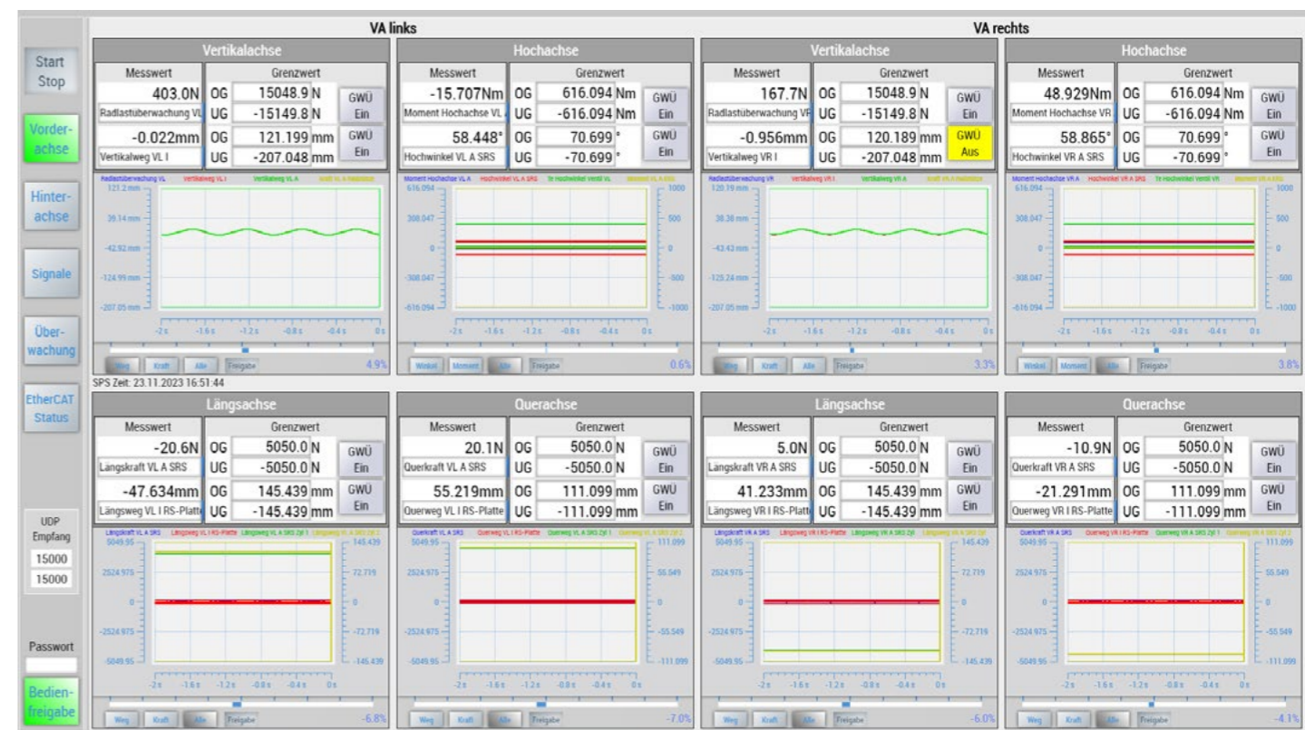
The measurements results can be visualized in detail with TwinCAT HMI.
