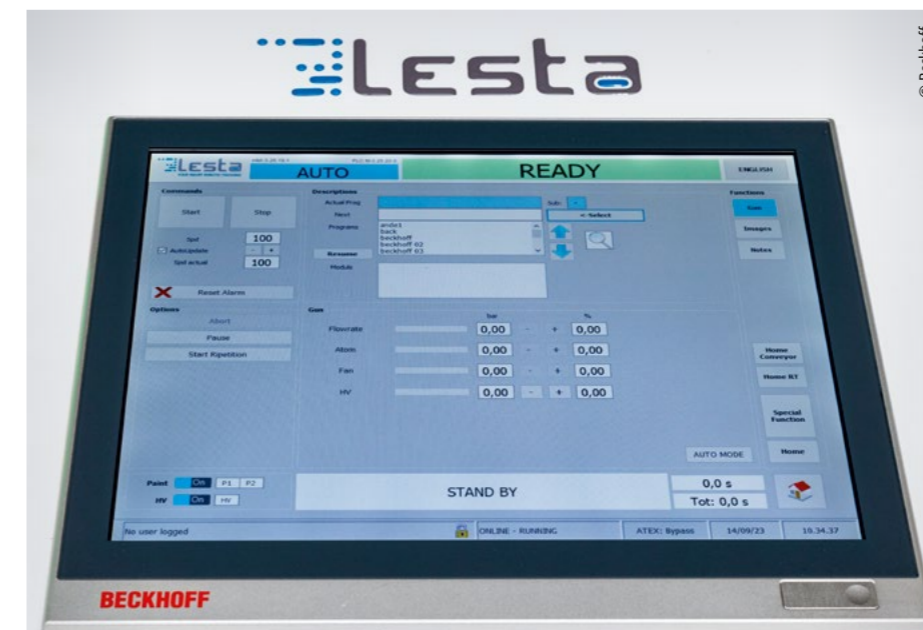
Lesta uses a CP2915 multi-touch built-in Control Panel to operate the painting systems.
