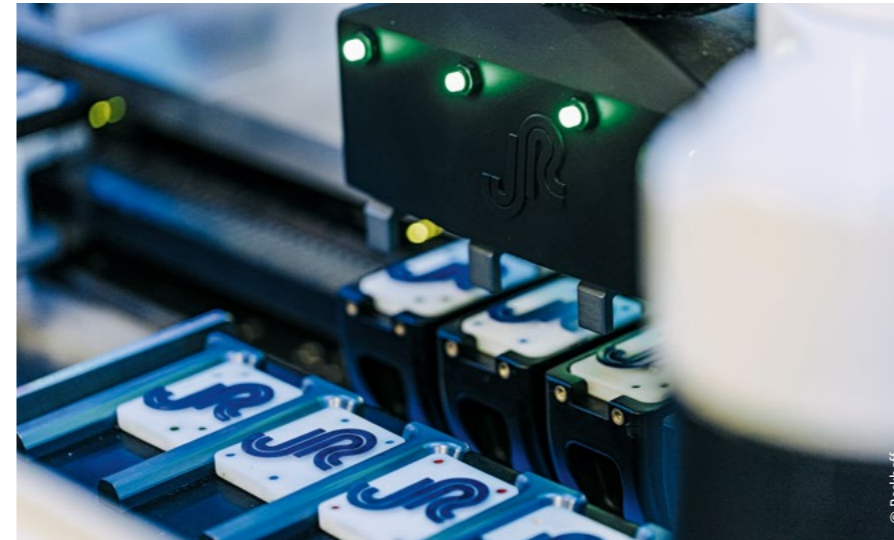
XTS movers can work synchronously or asynchronously, which is highly beneficial when processing multiple parts at the same time, for example, in the 4-up station shown here.
