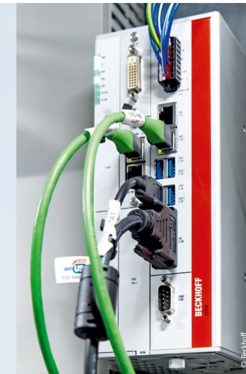
TwinCAT and a C6930 control cabinet Industrial PC handle the path control and coordination of all axes.
